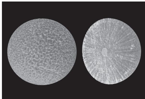
**Figure 5**  $\mu$ -CT rendering of the nucleus of the Brremangurey pearl, taken at 650  $\mu$ m radius from the centre void (left), with cut-away view showing the centre void and radial strut-like structures (right). Scanning was undertaken at 6.7  $\mu$ m resolution at 100 kV and 70  $\mu$ A.
