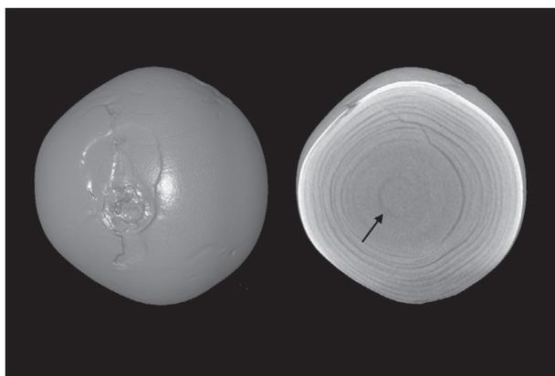
**Figure 4**  $\mu$ -CT surface rendering of the complete Brremangurey pearl (left) showing layers in cut-away view (right). Scanning was undertaken at 15  $\mu$ m resolution at 130 kV and 70  $\mu$ A. Pearl is 5.9 mm in diameter.
