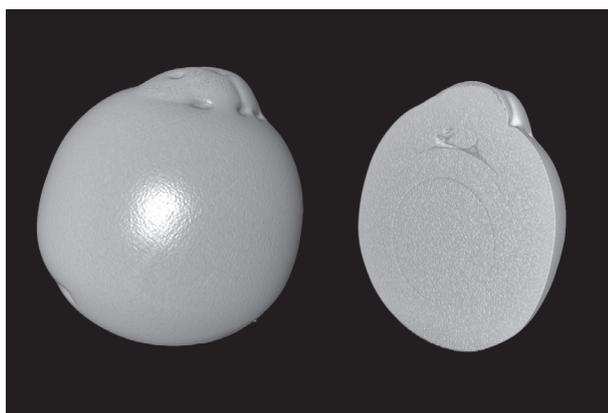
**Figure 3**  $\mu$ -CT surface rendering of a Cygnet Bay Pearl seeded in 2010 and recovered in 2012 (left) and showing two bands of nacre in cut-away view (right). An irregularity in banding has formed around an intrusive object during pearl growth. Scanning was undertaken at 31  $\mu$ m resolution at 130 kV and 70  $\mu$ A. Pearl is 10.6 mm in lateral diameter.
